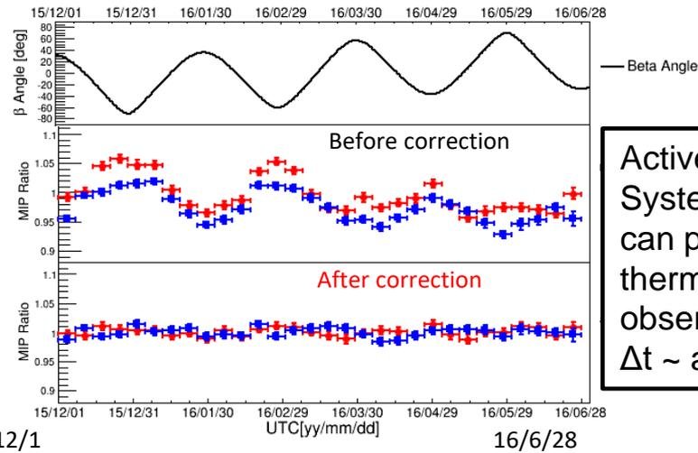
Active Thermal Control System (ATCS) on ISS can provide very stable thermal condition during observations:
