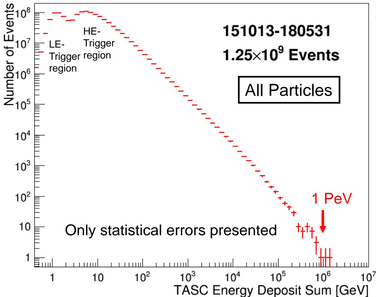
The TASC energy measurements have successfully been carried out in the dynamic range of 1 GeV – 1 PeV.
