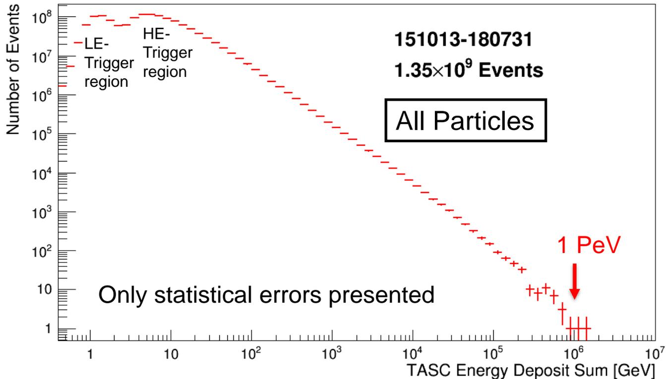
The TASC energy measurements have successfully been carried out in the dynamic range of 1 GeV – 1 PeV.
