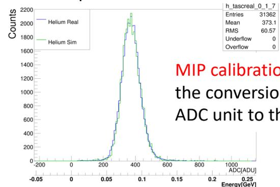
MIP calibration determines the conversion factor from ADC unit to the energy
