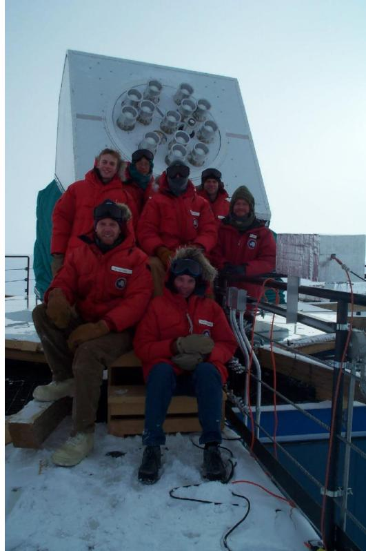
図 5.11: DASI is a 13-element interferometer designed to measure anisotropy of the Cosmic Microwave Background (CMB) Radiation over a large range of scales with high sensitivity. The instrument uses cooled HEMT amplifiers running between 26-36GHz, in ten 1 GHz channels and operates from the NSF Amundsen-Scott South Pole station. (<http://astro.uchicago.edu/dasi/>)
